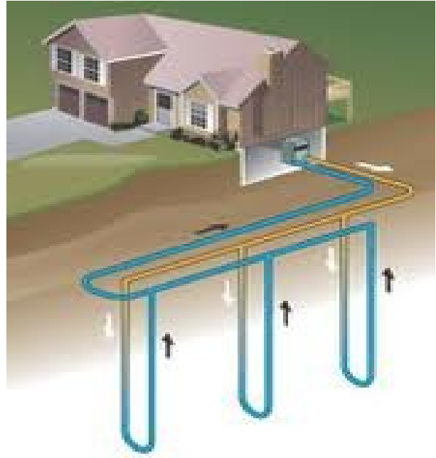
Figure 8. “Ground Source” system showing entry to Structure for a vertical closed loop systems .
